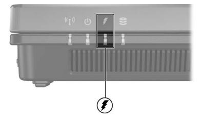
It is recommended that you leave the notebook connected to external power until the battery pack is fully charged and the battery light is turned off. A partially charged new battery pack can run the notebook after software setup is complete, but battery charge displays will not be accurate until the new battery pack has been fully charged.
